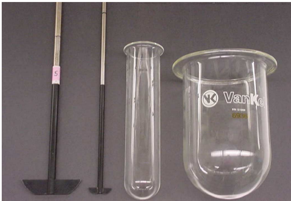
Fig. 1. Comparison of the USP Apparatus 2 vessel and paddle and the 200 ml conversion kit manufactured by VanKel Technologies, Inc.
